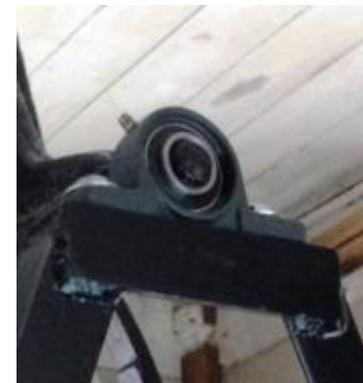
New sealed bearings for easy “pealing”.
